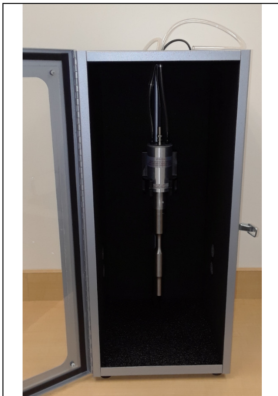
Example of the air cooling hoses set up properly with the enclosure.
